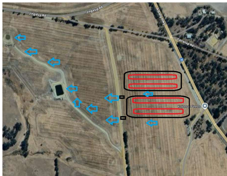
Figure 4. Water Overflow Movement Showing Dam 1 (Primary) and Dam 2 (Secondary)
